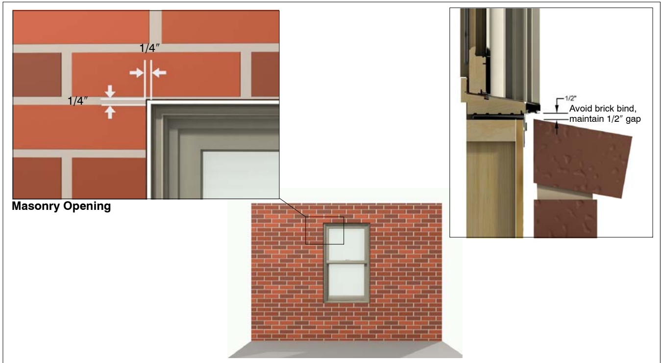
Figure 2: Typical rough and masonry openings.
