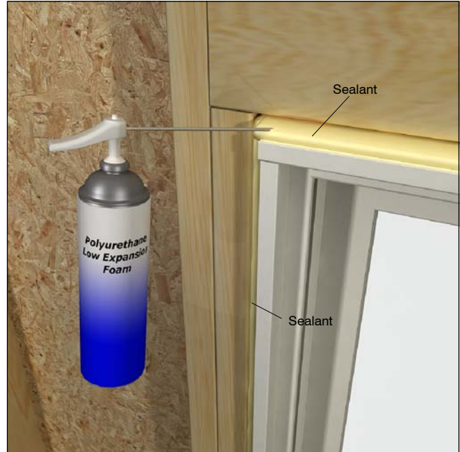
Figure 14: Apply low expansion foam between frame and rough opening
