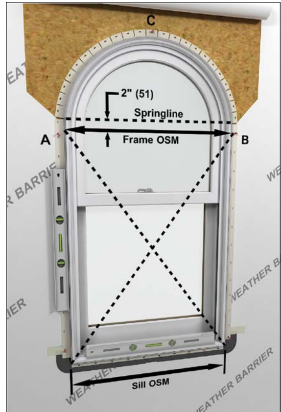
Figure 16: Shim and secure
