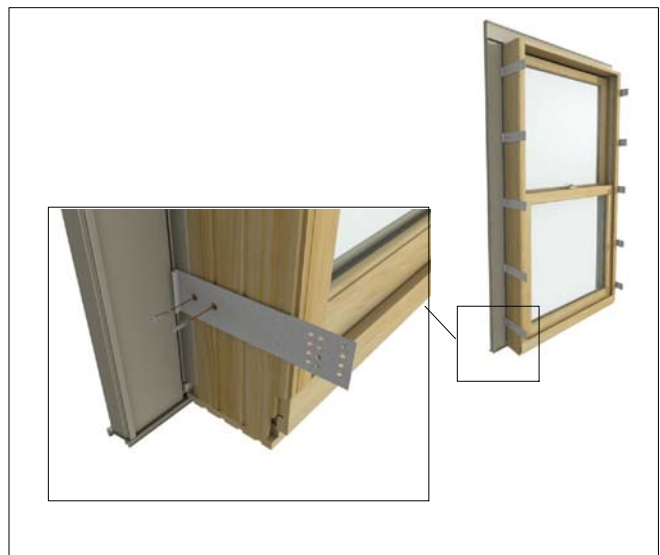
Figure 6: Apply brackets/clips to units with flat casing (if applicable)
